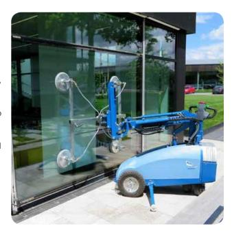
For example, the Clad-Lift 350 is designed to handle glass, windows, panels, doors or other elements up to 350 kg in weight with great efficiency. This vacuum lifting device with hydraulic telescopic beam enables the operator to rotate the workpiece by 360 ° vertical and 180 ° horizontal.;
