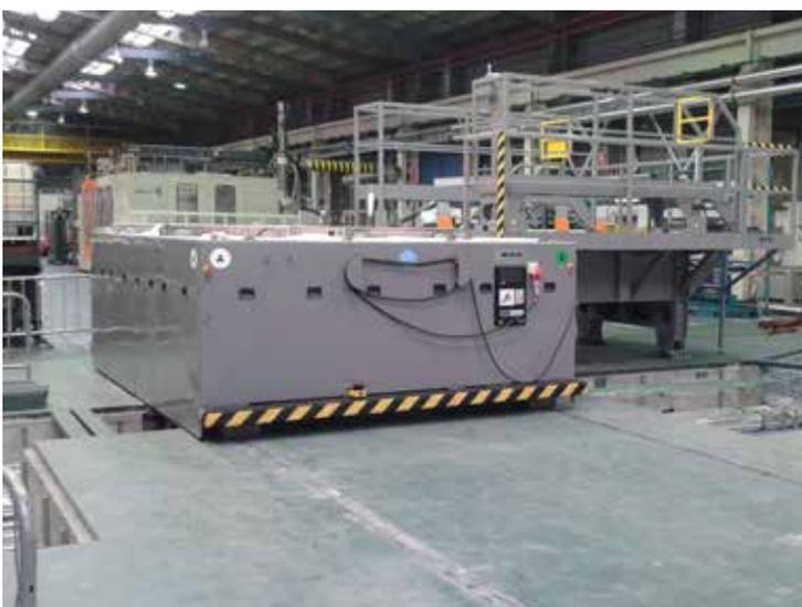
*EAS changes systems tables and cars are built up from a modular design. Moldweight range from 5 t till 100 t. EAS installation at the customer.*
