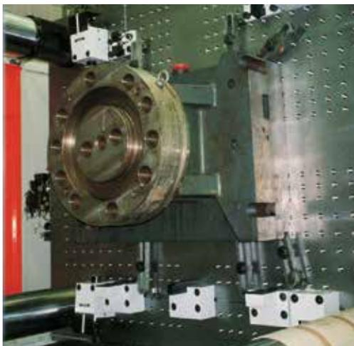
Drop and rotate solution with safety latches (the mold on this machine is just for testing)
