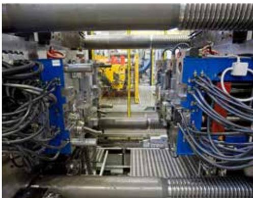
**Integrated hydraulic mold clamping systems EAS Engel**
