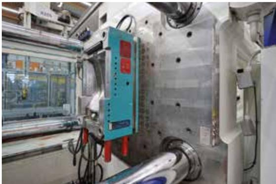
Pressmag SP on a 4000 kN (400 t) machine
