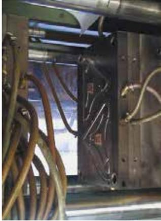
*Here is an example of the correct way of connecting several fluid circuits, without the risk of leakage or misconnection. When used in conjunction with a good water treatment system, EAS multi couplers will reduce scrap and improve the quality of your production.*
