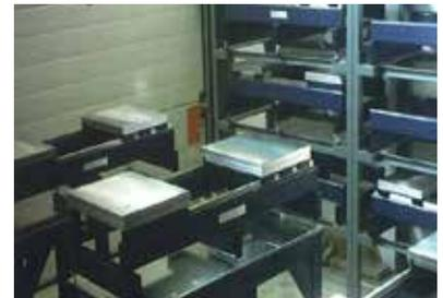
The standard units are all 1200 mm long, 580 mm wide and 275 mm high. The two turning platforms are 350 x 500 mm. Optionally the units can be placed on a higher table for easier access or if you have other requirements such as clamping solutions.
