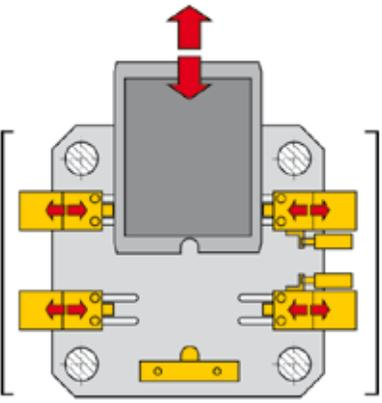
Vertical load mould change solution with, movable clamps. Clamps are moved manually or with hydraulic cylinders.
