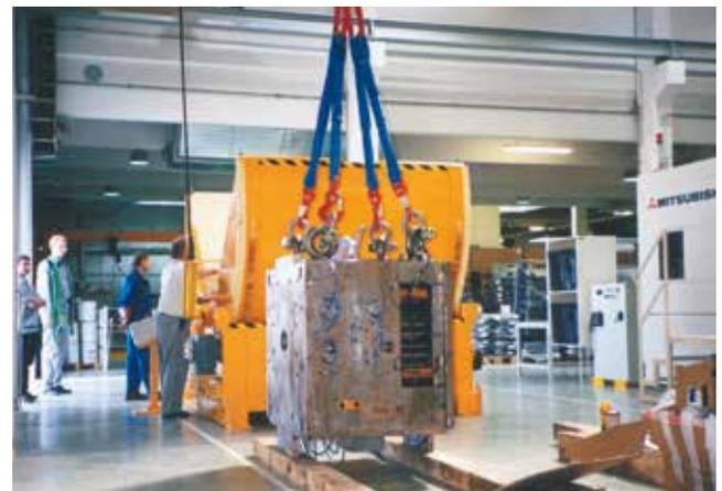
*This turning unit is for molds up to 20 t and is remote controlled. EAS can supply these units up to 100 t mold weight.*
