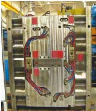
*Two standard manual multi couplers with 12 water connections, a special manual multi coupler with 5 electric connectors for signals and heating purposes and one special manual multi coupler for hydraulic core pulling connections are mounted on these 40 t molds.*
