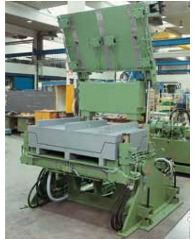
*MOD wedge clamps were integrated in a specially designed ring for this special "Ringwalz" machine to produce automotive wheel frames. Due to the self-locking feature of this clamp, hydraulic pressure is not required after clamping or during the rotational movement of the ring.*
