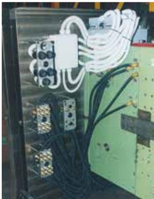
*A manual multi coupler with several electrical connectors for heating and sensor signals. A standard 12 connection multi coupler, with size 12 (1/2") water connections is used for the cooling circuits. A park station is used for hanging the manual multi coupler during mold change. These multi couplers solutions were implemented on five 1300 t machines.*
