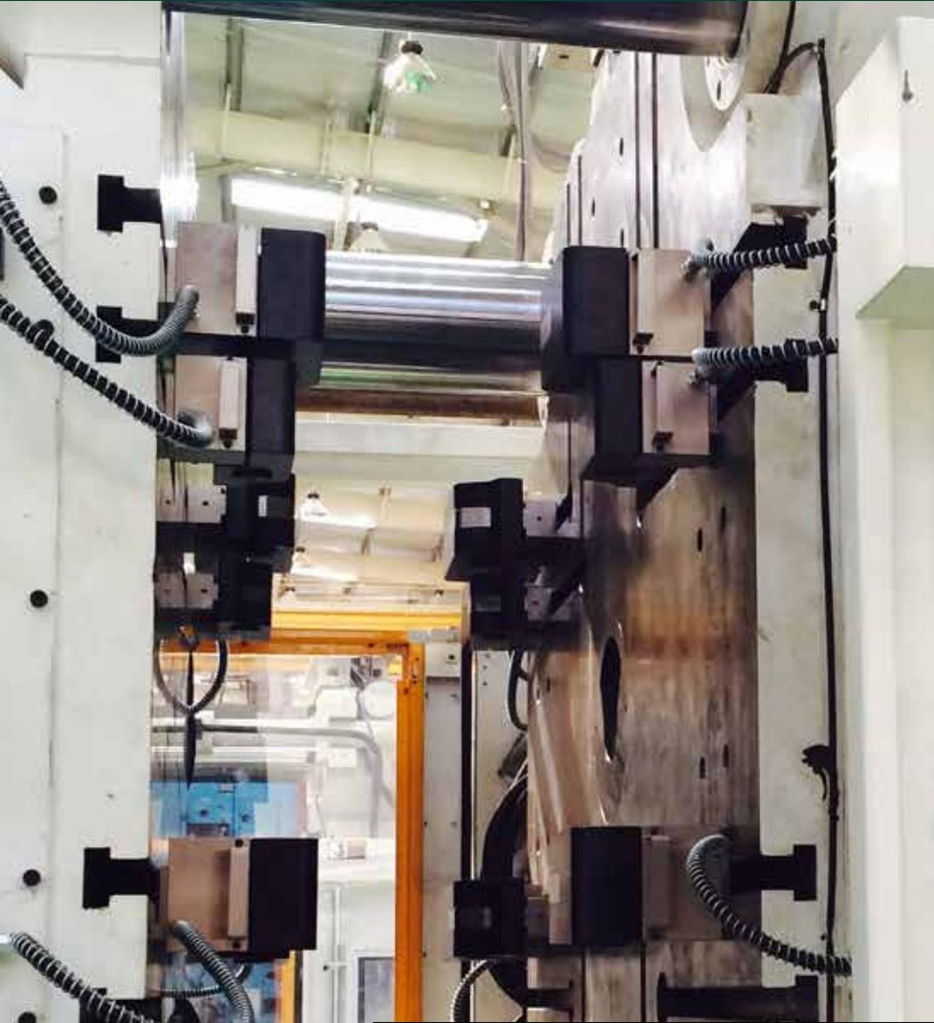
Single acting ERC cylinders can be powered by the EAS air hydraulic pump units with on each plate 2 circuits for safety purposes.
