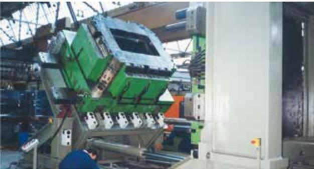
For a well known German manufacturer of plastic containers EAS equipped several large injection molding machines up to 6000 t with an adaptive hydraulic clamping systems, an air cushion mold change car, several mold storage racks and an inspection unit for molds up to 100 t.
