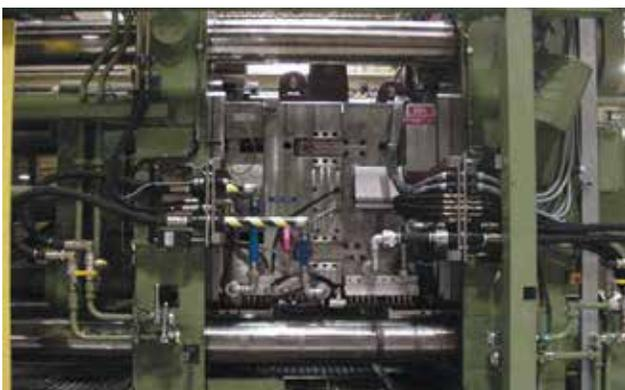
*Large size 37 mono couplers are part of the multi couplers on this machine to connect leakproof large cooling lines. This in combination with heating oil connections and electric connections results in a total mold change time of less than 15 minutes in combination with hydraulic clamping and a vertical mold change by means of an overhead crane on this 2300 t machine. Fast, safe and clean.*
