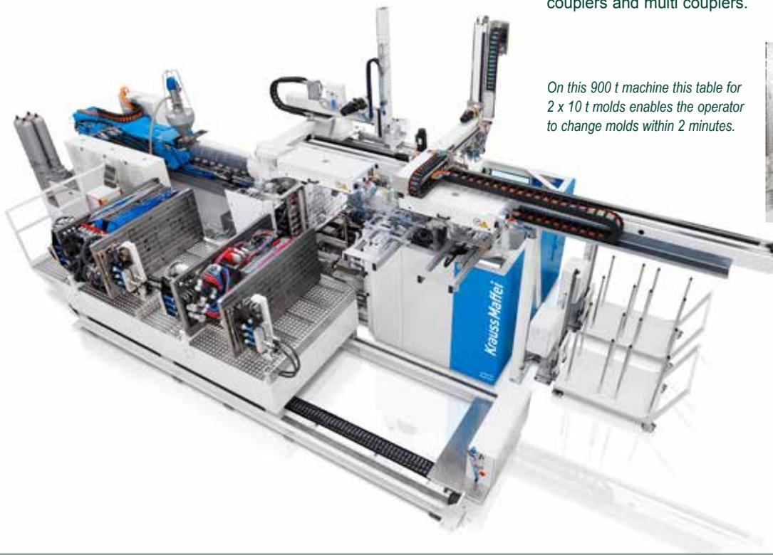
On this 900 t machine this table for 2 x 10 t molds enables the operator to change molds within 2 minutes.
