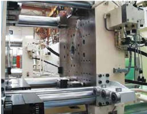
Powered roller system on a 500 t machine
