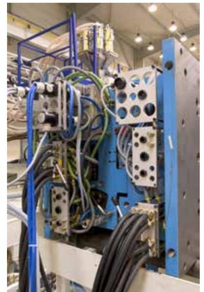
*This is an example of how fluid connections are often done, resulting in inefficient cooling, leakage and high scrap rates.*
