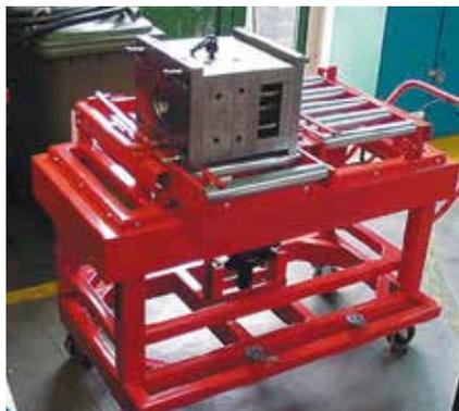
*The molds are pushed and pulled manually.*
