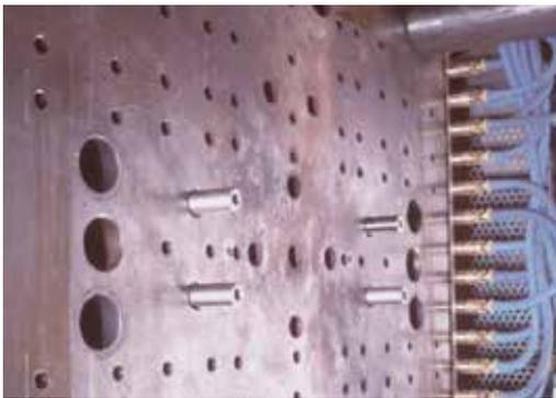
**For machines with American SPI platen configuration EAS has designed SPI ejector couplers which can be used with the 1" and 2" SPI ejector patterns without platen modification.**
