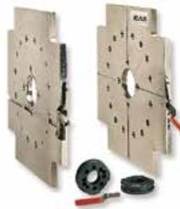
Manual clamping solutions are available for SPI machines with multiple ejector bar holes. These systems utilize a rack and pinion to rotate the lock ring to clamp the mold in place. The SPI manual clamp systems are equipped with removable handles. SPI clamping plates have a thickness of 1" inch. Bayonet adapter rings are available in a variety of configurations.
