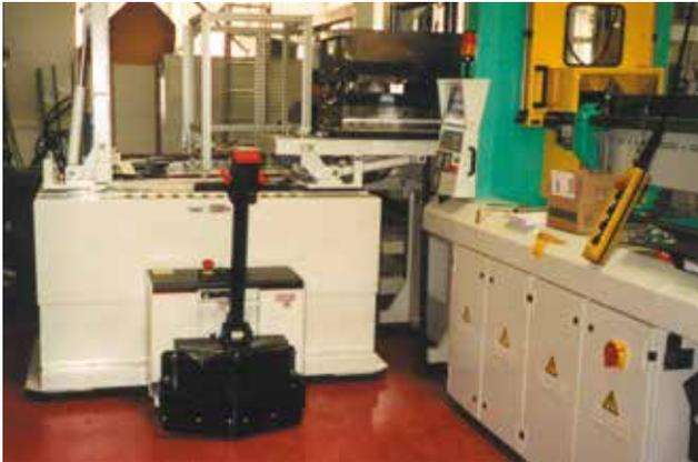
**A special electrically driven mold change car for molds up to 1700 kg is also used as an inspection unit.**
