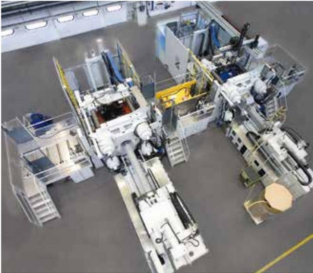
**Single station mold change tables at each side of the injection molding machine with driven rollers on the table and in the machine provide very fast and automated mold changes.**
