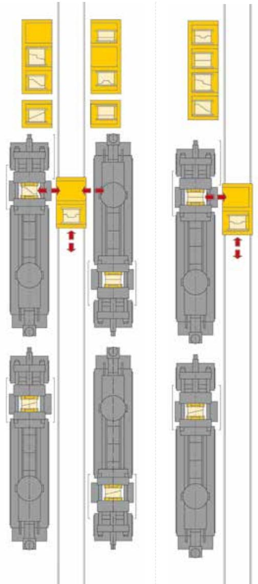
*Mold change car travels within rows of machines and storage systems and pre-heating stations, changing to both sides of the car.*
