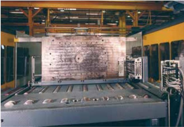
**When using a mold change table between two injection machines you will improve your return on investment because the table is supporting two machines instead of one. This provides greater flexibility and faster changeover.**
