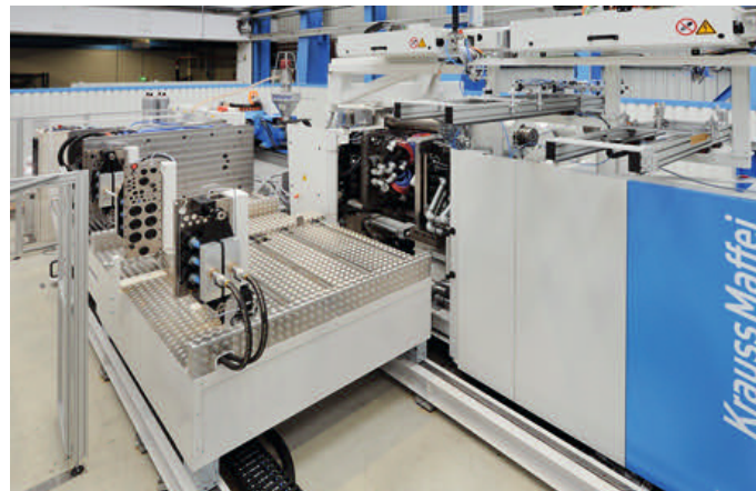
Fig. 2. The mold double shuttle table is in the transfer position for automatic mold removal. In the preheating station 2, the next mold has already been brought to the operating temperature (figures: KraussMaffei/EAS)
