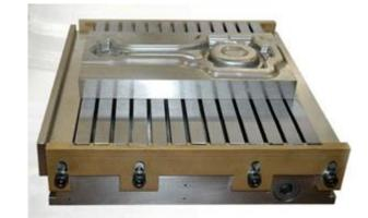
The Neopower chuck is a new concept for use on (high speed) milling machines, finishing operations, or for tool/die applications, allowing to hold, raise and support the workpiece effectively, even without back or end stops. A high milling accuracy can be achieved thanks to the high holding power in conjunction with the low magnetic field. Clever accessories and a modular design allow for quick set up and a great flexibility.
